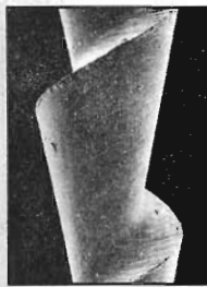
Figure 5. Hedstrom file (Maillefer) x 150. With a helical angle of approximately 70 degrees.
